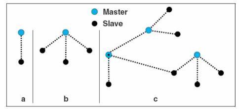
Piconets with a single slave operation (a), a multi-slave operation (b) and a scatternet operation (c).
